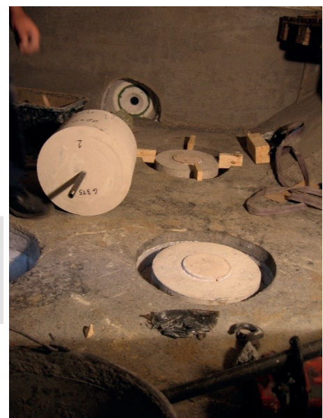
Installation of gas diffusers in an aluminium melting furnace.
